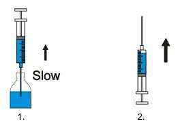
3. Connect a blue-striped PEEK (250 μm ID, 1/16" OD, typically 45 cm in length) inlet tubing to the syringe using a Luer lock connector. Fill the inlet tubing with sample solution.
